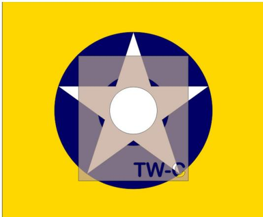
The final "C" mask for the insignia Red should be applied using the 5 registration cut outs which align with the internal corners of the star. With these marks evenly seated the circle should be positioned perfectly in the centre. Use minimum pressure initially so the masks can be easily lifted and re-positioned if necessary.
