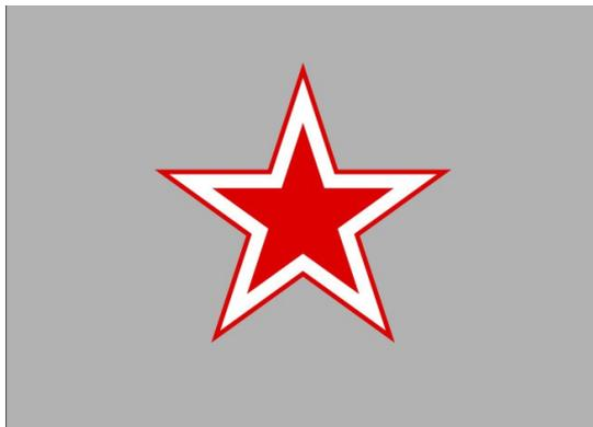
For each complete marking there are 2 masks involved. One is for the main Red star which is applied first, and the second is for the white inset border.
